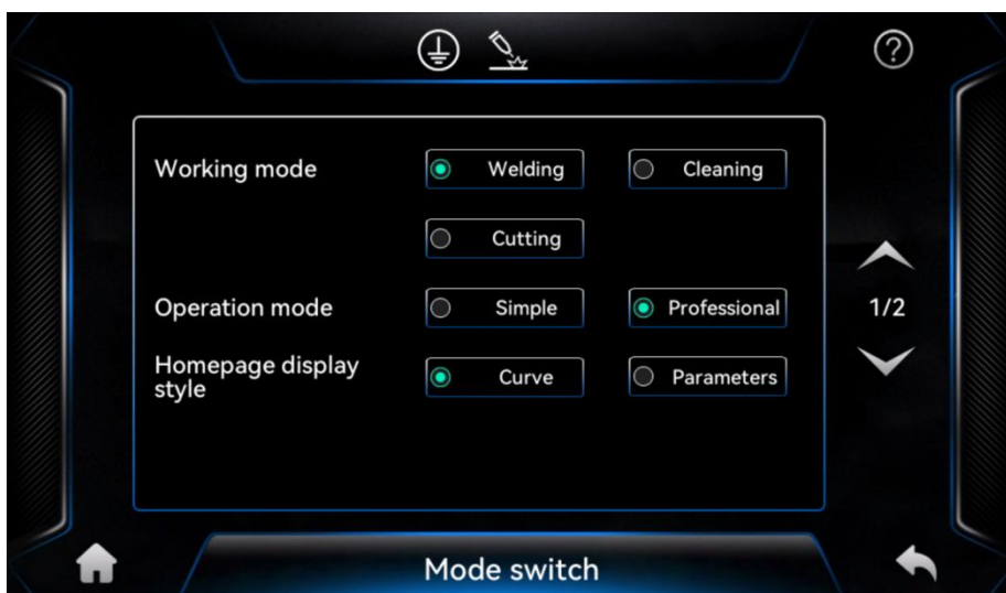
Figure 3-22 Control Panel • Settings Page • Mode Switching • Page 1
