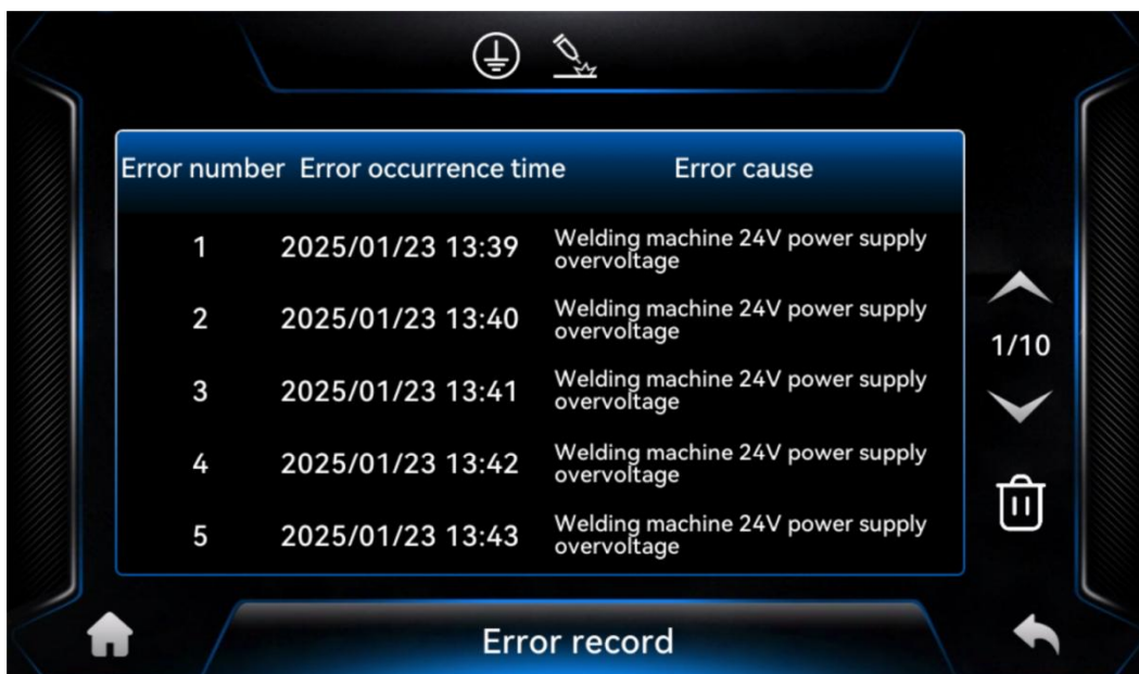
Figure 3-17 Control Panel • Settings Page • System Parameter • Fault Record
