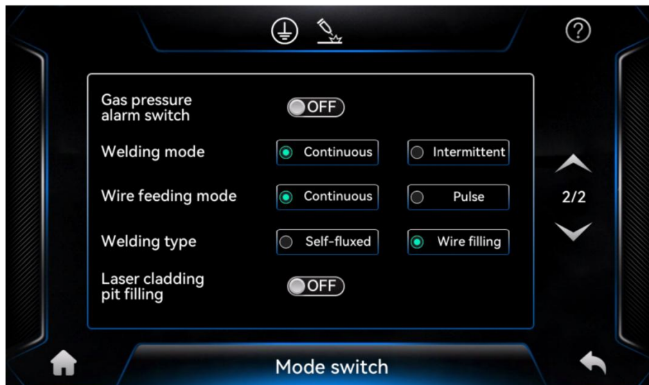
Figure 3-23 Control Panel • Settings Page • Mode Switching • Page 2
